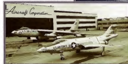
▶ Flaps down The Voodoo was built to fly very fast, but its large split flaps and leading-edge flaps gave it good handling at low airspeed, even when fitted with large external fuel tanks.
